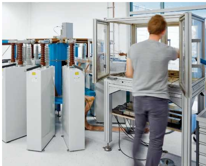
Fig. 27: Lightning surge current generator
