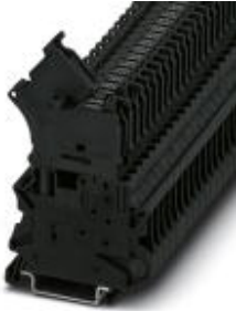
Lever-type fuse terminal block, black, for 5 x 20 mm G fuse inserts, with LED for 250 V AC
