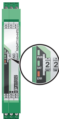
Figure 7-13 Diagnostic LEDs of the RAD-PT100-4-IFS
