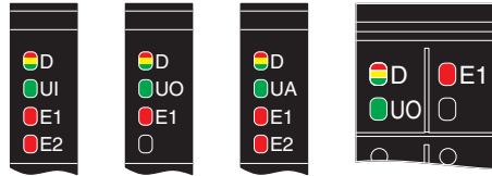
Figure 10-2 LEDs on the power connectors (examples)
