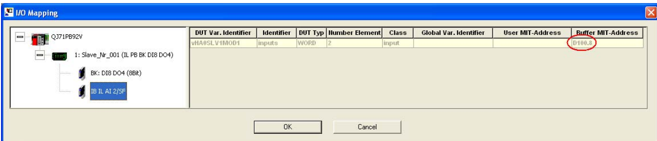
Figure 3-2 I/O assignment of analog inputs (odd byte address)
