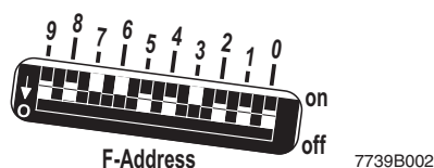
Figure 2-9 Switch for F_Destination_Address (F_Dest_Add)
