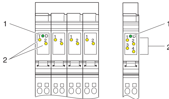
Figure 9-2 Indicators on I/O terminals
