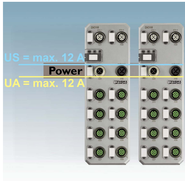
Figure 4-13 Voltage feed U_S and U_A
