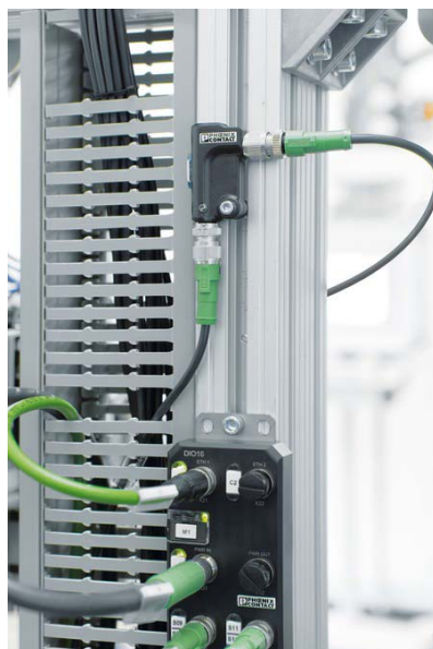
Figure 5-7 IO-Link/analog converter and Axioline E IO-Link master
