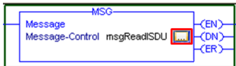
Figure 5-14 Opening the configuration field
