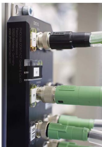
Figure 4-11 Axioline E device with connected M12 connectors
