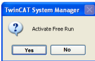
Figure 4 Activate "Free Run"
