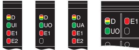
Figure 10-2 LEDs on the power connectors (examples)
