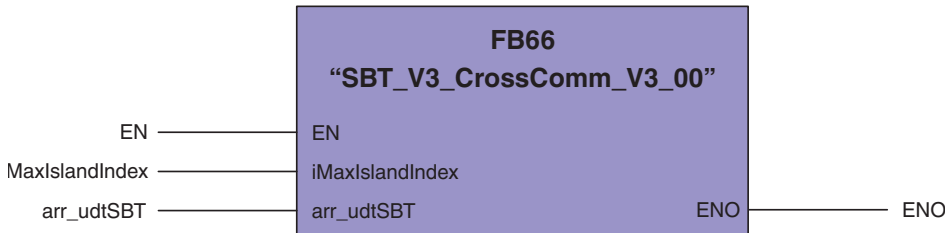
Figure C-2 “SBT_V3_CrossComm_V3_00” function block (FB66)
