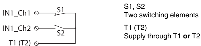
Figure 7-14 Two-channel non-equivalent assignment of inputs, supply through T1 (or T2), cross-circuit monitoring disabled
