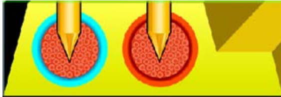
Figure 4-9 Cable connection using the penetration technique
