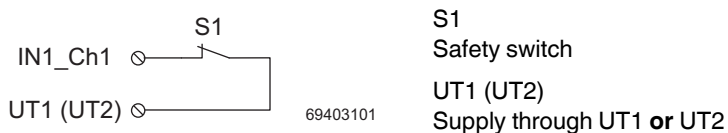
Figure 7-2 Single-channel assignment of inputs: Supply through UT1 or UT2 (clocking disabled for each)
