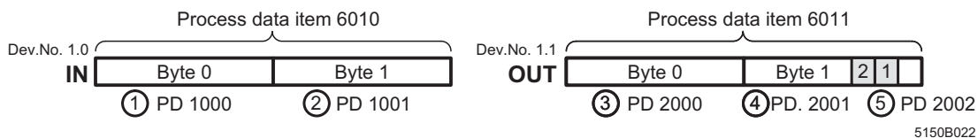
Figure 1-21 Byte IN and OUT process data
