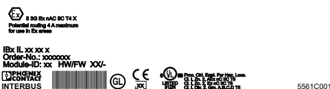
Figure 2-6 Typical labeling of terminals for use in potentially explosive areas
