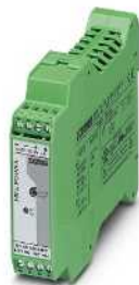
Input: 85 ... 264 V AC, 90 ... 350 V DC MINI-PS-100-240AC/5DC/3 Order Number: 2938714
