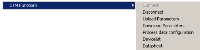
Figure 17-20 DTM functions of the IB IL IFS-MA-PAC
