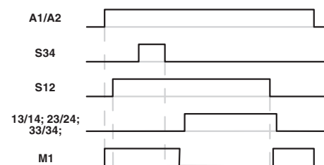
Figure 2 Time diagram for manual, monitored start
