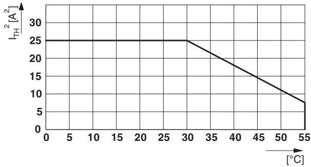
Figure 2 Derating curve - any mounting position, without spacing
