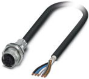
Flush-type socket, shielded, 5-pos., M12, A-coded, rear/screw mounting with M16 thread, with 2 m cable, 5 x 0.34 mm 2
