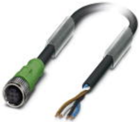
Sensor/actuator cable, 4-position, PUR, black-gray RAL 7021, free cable end, on Socket straight M12, A-coded, cable length: 5 m
