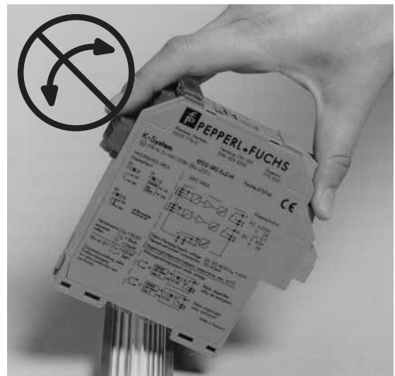
INCORRECT: Unit snapped on at an angle.
