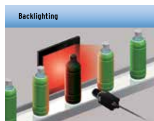
External shape inspections
