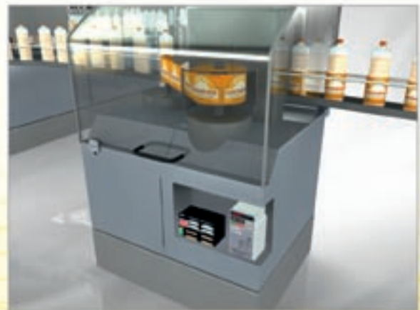
Safe shutdown is controlled by a Safety I/O-Module, additionally monitoring safety door switches.
