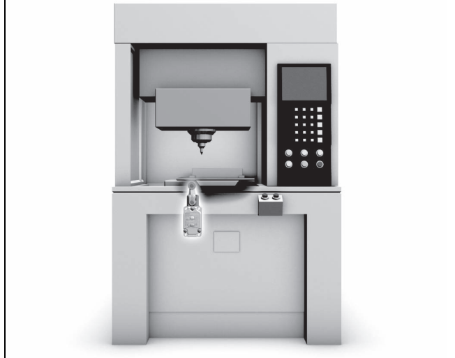
Detection of Work Table Origins (X, Y, and Z) on Machine Tools
