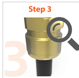
The backnut should be level with the marking guide corresponding to its diameter – this can be visually inspected and adjusted as necessary
