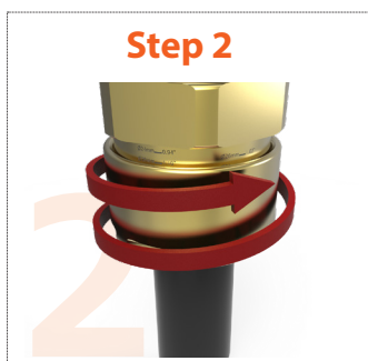
Tighten backnut until a seal is formed onto the cable, then tighten one further turn
