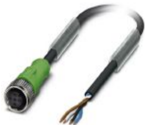
Sensor/actuator cable, 4-position, PVC, black RAL 9005, free cable end, on Socket straight M12, coding: A, cable length: 3 m
