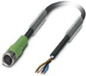
Sensor/actuator cable, 4-position, PVC, black RAL 9005, free cable end, on Socket straight M8, cable length: 3 m
