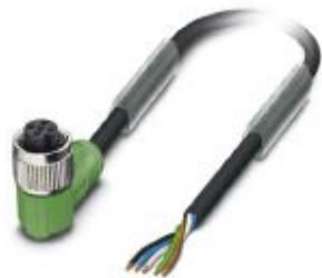
Sensor/actuator cable, 5-position, PVC, black RAL 9005, free cable end, on Socket angled M12, coding: A, cable length: 10 m
