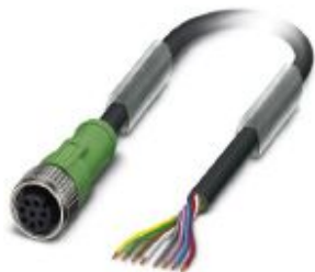
Sensor/actuator cable, 8-position, PVC, black RAL 9005, free cable end, on Socket straight M12, coding: A, cable length: 3 m
