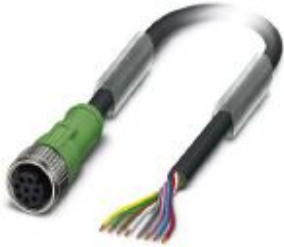
Sensor/actuator cable, 8-position, PVC, black RAL 9005, free cable end, on Socket straight M12, coding: A, cable length: 10 m
