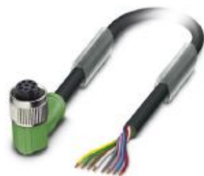
Sensor/actuator cable, 8-position, PVC, black RAL 9005, free cable end, on Socket angled M12, coding: A, cable length: 10 m
