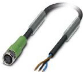
Sensor/actuator cable, 3-position, PVC, black RAL 9005, free cable end, on Socket straight M8, cable length: 5 m
