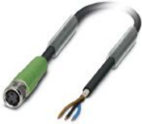
Sensor/actuator cable, 3-position, PUR halogen-free, black-gray RAL 7021, shielded, free cable end, on Socket straight M8, cable length: 3 m
