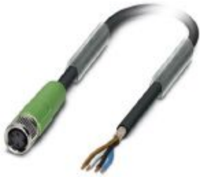
Sensor/actuator cable, 4-position, PUR halogen-free, black-gray RAL 7021, shielded, free cable end, on Socket straight M8, cable length: 5 m
