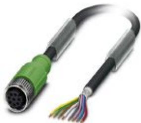
Sensor/actuator cable, 8-position, PUR halogen-free, black-gray RAL 7021, shielded, free cable end, on Socket straight M12, coding: A, cable length: 3 m
