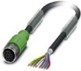
Sensor/actuator cable, 8-position, PUR halogen-free, black-gray RAL 7021, shielded, free cable end, on Socket straight M12, coding: A, cable length: 20 m
