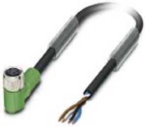
Sensor/actuator cable, 4-position, PUR halogen-free, black-gray RAL 7021, free cable end, on Socket angled M8, cable length: 3 m
