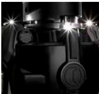
4 LED lighting of the working area
