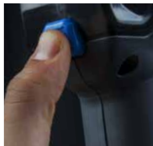
Manual pressure release button
