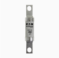
Fuse-link, LV, 40 A, AC 500 V, BS88/A4, 25 x 110 mm, gL/gG, BS
