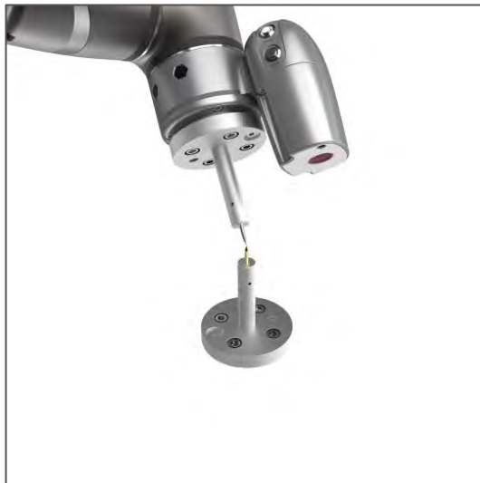
Figure 111: The Robot Posture Needs to Change during Teaching (1/2)
