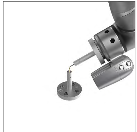
Figure 111: The Robot Posture Needs to Change during Teaching (1/2)
