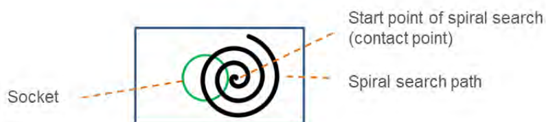
Figure 226: Spiral Searching Method
