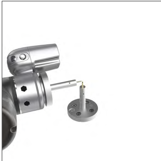
Figure 112: The Robot Posture Needs to Change during Teaching (1/2)
