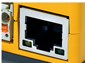
Ethernet interface Modbus/TCP and REST API, transfer of permissions and access to web server
